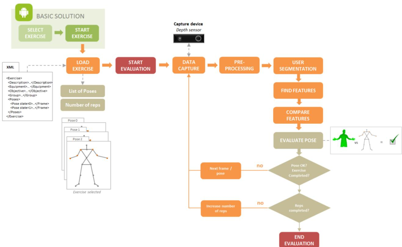
Figure 3.2 . Functioning of the 3D Motion Sensing module
