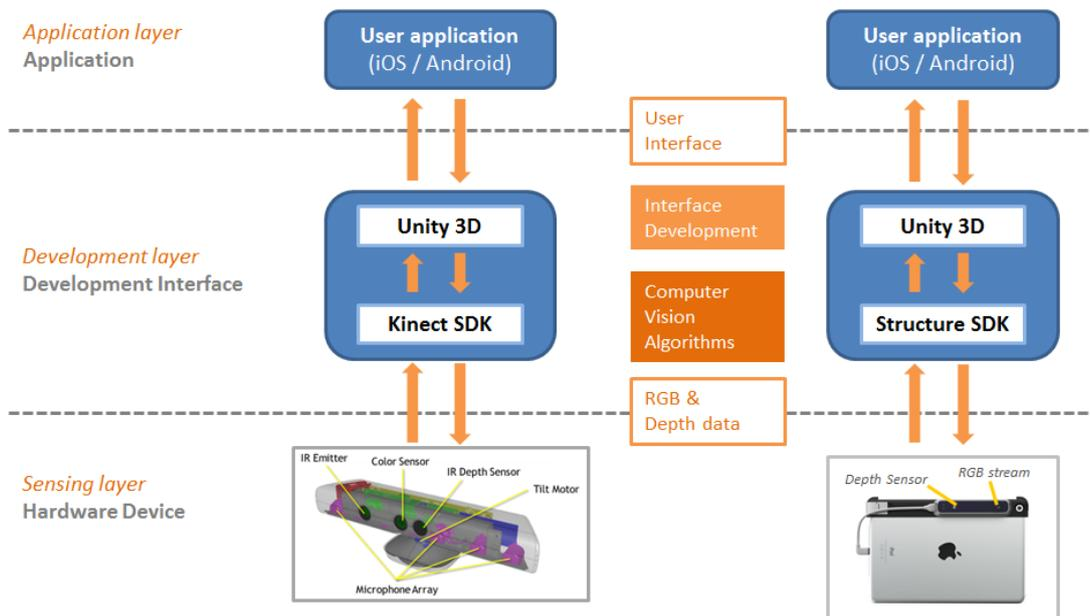
Figure 3.1 . Module diagram for Kinect and Structure sensors
