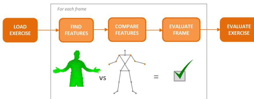
Figure 3.5 . Functional blocks of the 3D Motion Sensing module (II)
