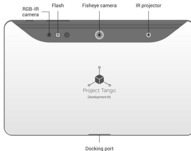
Figure 2.2 . Hardware Diagram for the Tango Tablet Development Kit
