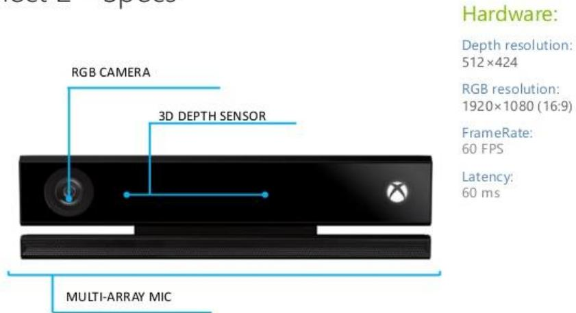
Figure 2.5 . Kinect 2 sensor
