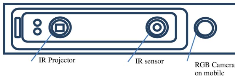
Figure 2.3 . Hardware Diagram for the Structure Sensor device
