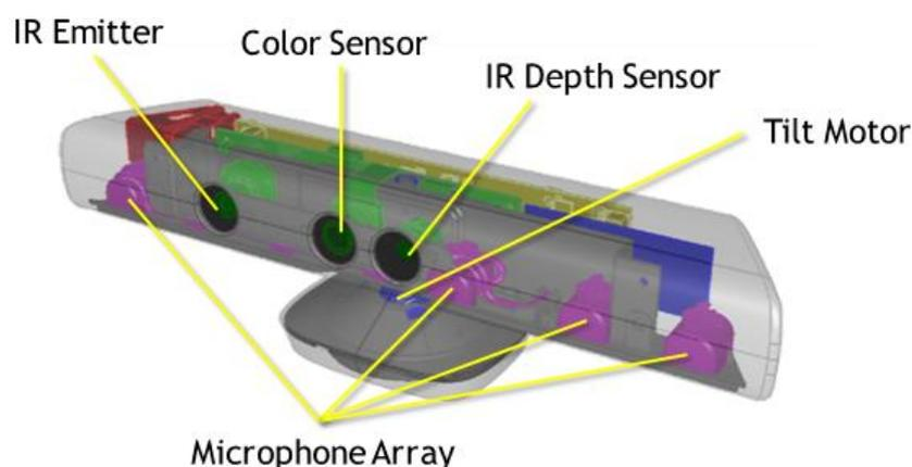
Figure 2.4 . Kinect sensor
